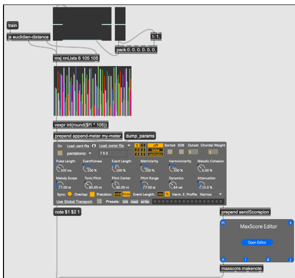
Figure 12. Metric interpolation performed by the nnLists object, a simple MLP object with one hidden layer. Parameter settings—including the stored tonal-semblance and metric profiles—are sent as dictionaries to the DJster Scorepion, a MaxScore Editor plugin via the dump_params message.
